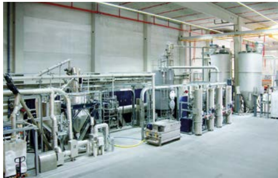
Using the new VACUNITE® system, the RCS Group is expanding their plastics recycling division to include the production of food-grade PET recyclate for food and beverage packaging, films and blisters.
