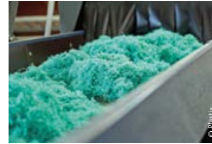
Only when the residual materials have been separated, shredded and washed in the purest possible way in terms of type and colour are they transferred to the regranulation line.
