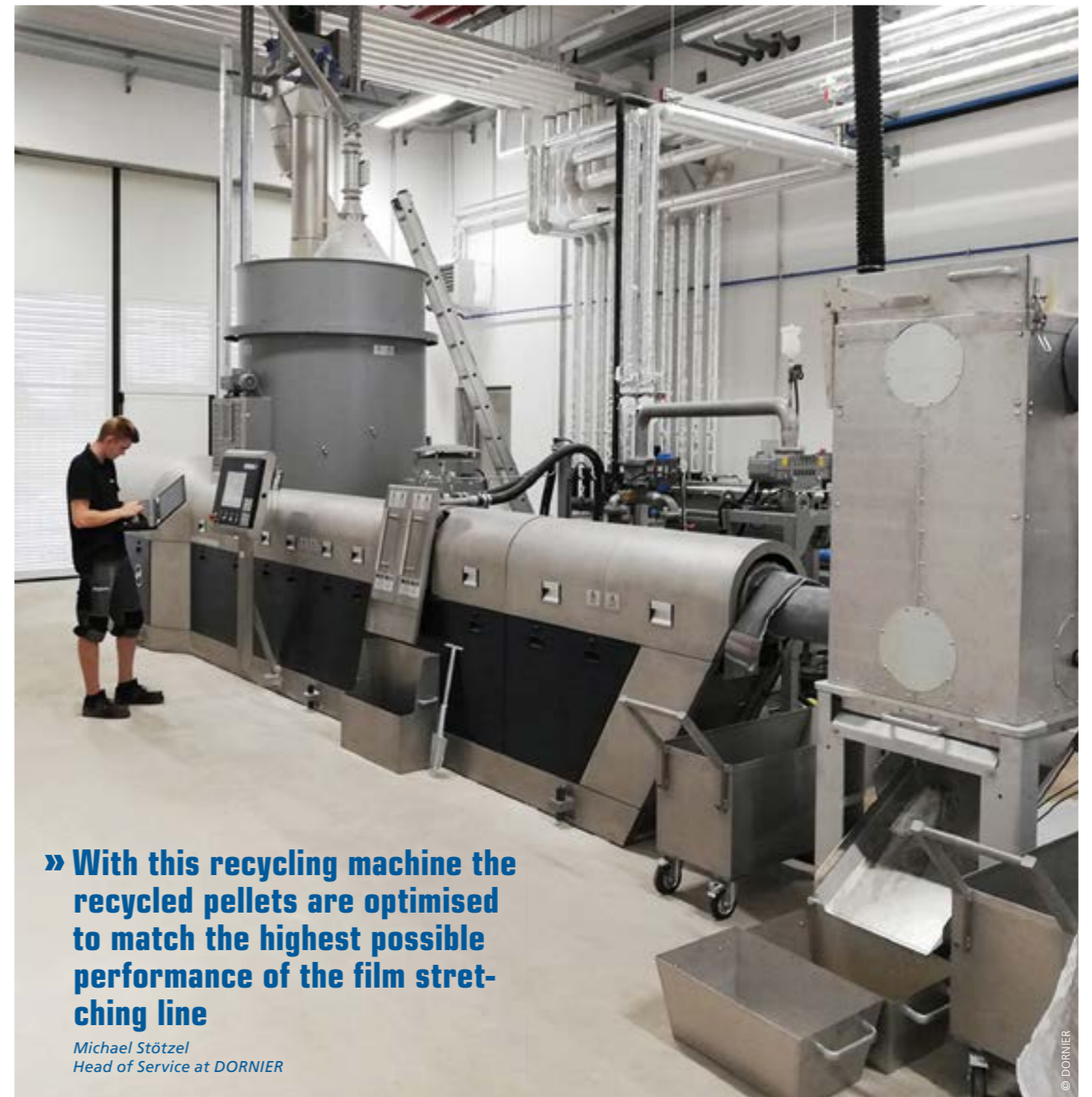
The recycling system is an application-specific combination of an INTAREMA® 1512 TE recycling machine with a Lindauer DORNIER melt filter for fine filtration.
