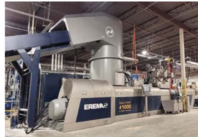
Picture above: PreZero US uses the new EREMA machine at its facility in South Carolina for processing washed LDPE flakes. .
