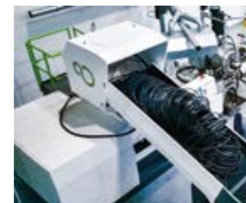
As an all-rounder, the ISEC evo machine processes bulky hose bundles as well as start-up lumps and complete rolls with drip tapes.
